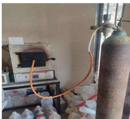
Muffle Furnace with Nitrogen Cylinder
