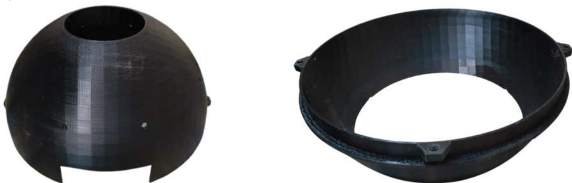
Figure 4 Top cover Bottom cover of the housing of the robot
