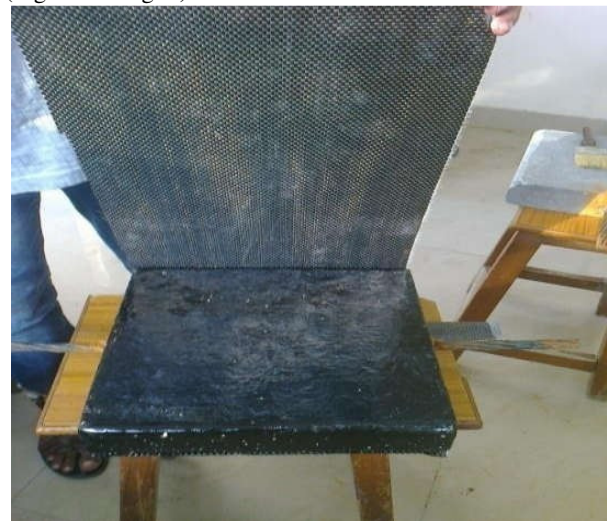
Fig. 2 Wrapping of FRP sheet after coating Epoxy paint [10].
