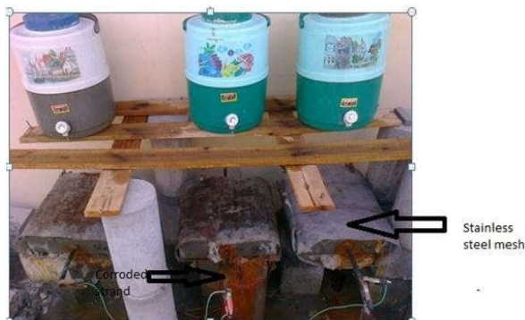
Fig. 1 Block Specimen subjected to 5% NaCl Solution [10]
