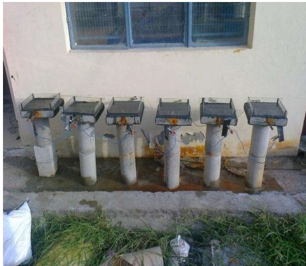
Fig. 4 Set up of slab specimens for Active Protection [10]
