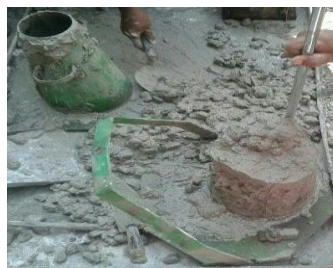
Fig. Testing of slump cone
