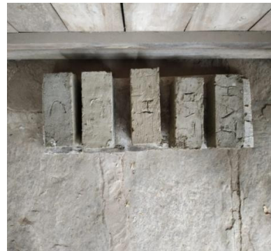
Fig. Drying of brick
