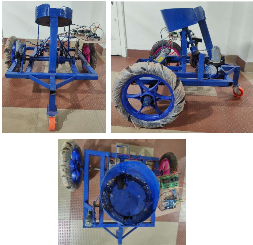
Figure 7. Variable distance seed sowing machine using Arduino
