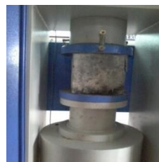
Figure Compressive strength test
