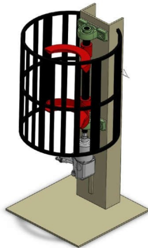
Figure 8: An isometric view of the Spring compressor
